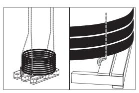
If chains are used exclusively, they are placed under the pallet as appears from the illustration.
