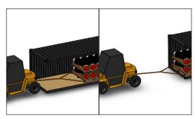
1. Pull the pallet with the goods to the edge of the container, using straps.
