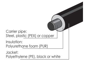
The pipe dimensions are indicated as follows: 76,1 mm / 140 mm
