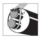
As for 12 m pipes the straps can alternatively be placed as appears from below illustrations. The straps are placed on the outmost third of the pipe end. It is vital to ensure that the straps do not get in contact with the jacket.
