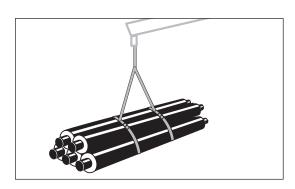
The pipe bundle is lifted off the lorry trailer by means of the straps.
