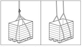
When unloading pallets place the straps under the pallet in one of the following two ways.
