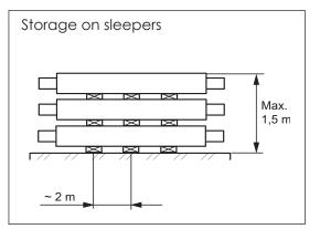
The best method of storing straight pipes is to lay them on an even and solid substratum of stonefree sandbanks with a minimum width of 0.5 m and a max. distance of 5 m as illustrated.
