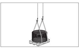
Place the straps under the pallet without the straps getting in contact with the coil.
