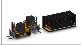
3. When enough of the pipe has been pulled out of the container, it is supported from the side by another forklift. Remove the strap.
