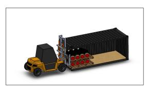
2. Lift the pallet safely, using a forklift or a loader, equipped with forks.
