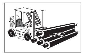
Carefully lift the pipes off the lorry trailer with the forklift.
